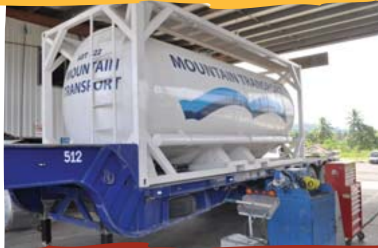
Specialist ISO Tanker used for the PJV Bulk Cement Haulage
